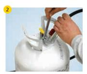
Hand-tighten hose fitting onto TurboStick cylinder. Avoid crossthreading the fittings which will result in leaks at the connection. Use properly sized open end wrench to tighten fitting. DO NOT OVERTIGHTEN.
