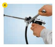
Hand-tighten hose fitting onto application pistol inlet fitting. AVOID CROSS-THREADING. Use properly sized open end wrench to tighten fitting. DO NOT OVERTIGHTEN.
