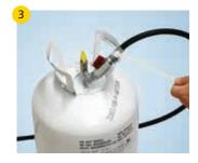
Verify the valve on the hose and the flow-control valve on the pistol are fully CLOSED. Secure hose to cylinder handle with plastic tie to protect hose and connection from incidental damage during use.
