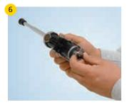
Open flow control valve on the back of pistol and dispense Turbostick material into an open container until steady flow and uniform consistency is achieved.
